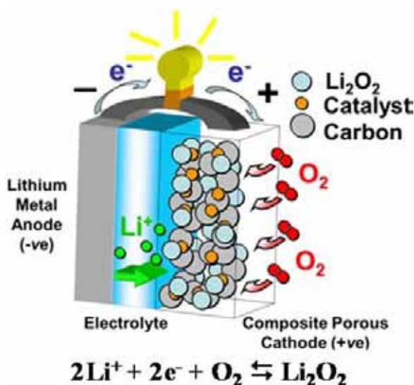
Figure 1. Non-aqueous rechargeable Li-O 2 cell
