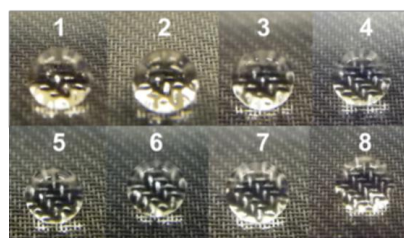
Fig. 2 Liquid droplets on the superoleophobic aluminum mesh surface: 1. rapeseed oil, 2. hexadecane, 3. dodecane, 4. acetone, 5. ethanol, 6. octane, 7. 2-propenol, 8. hexane.
