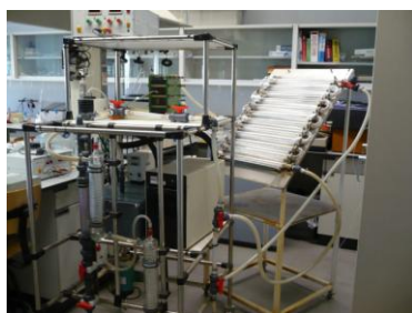
Fig. 1- Solar photoelectro-Fenton pre-pilot flow plant.
