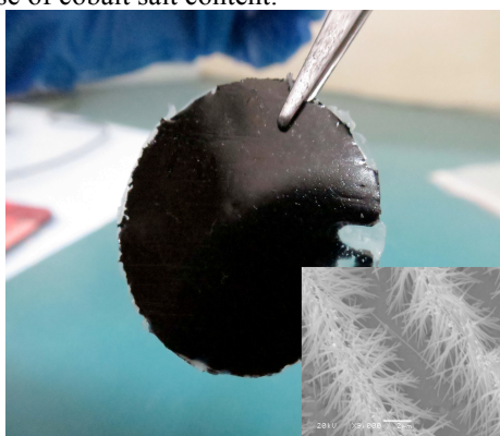
Fig.1. The digital photograph and the SEM image of Ni-Co NWAs electrode (inset); Fig.2. The performance of direct urea-hydrogen peroxide fuel cell. Open dots: CFC at both sides, solid dots: Ni-Co NWAs and Pd@CFC respectively.
