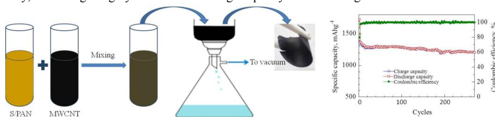
Fig 1. Schematic of the S/PAN/MWCNT binder free cathode preparation and it's cycleability at 0.2 C.
