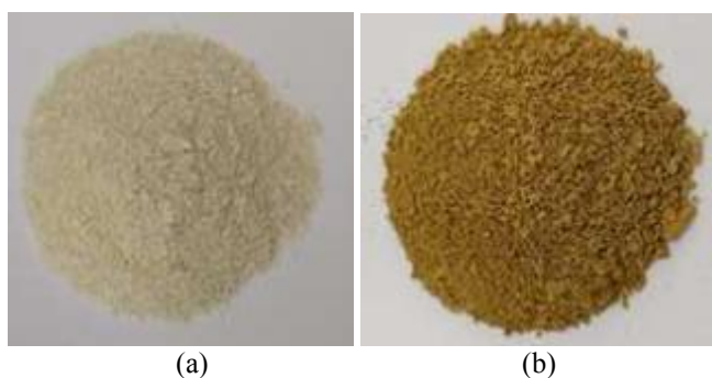
Synthesized Si nanoparticles (a) without and (b) with \text{H}_2 as swirling gas
