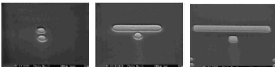
Figure: SEM images of nanoelectrode pairs; circular electrodes are 300 nm in diameter.
