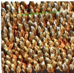
Fig. 2. Zn-Ni film deposited from liquid crystal; 1.6 x 1.6 x 0.08 $\mu$ m.
