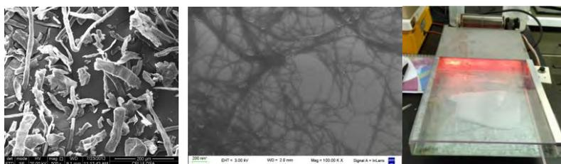
**Figure 1:** Sigma C8002 Alpha-cellulose (left), fibrillated NC (middle), casted NFC suspension (right)
